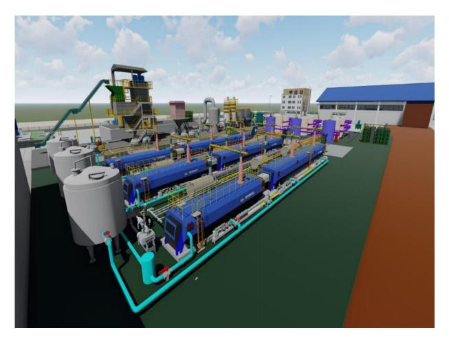
The existing thermal decomposition method is very economical because only chemical substances such as waste vinyl, plastic, and rubber can convert energy and require long-term heating at a high temperature of 1,000°C or higher. However, the CEP decomposition method is very economical because all combustible wastes are mixed and input at the same time and decomposed within minutes at 400~450°C to convert energy.
